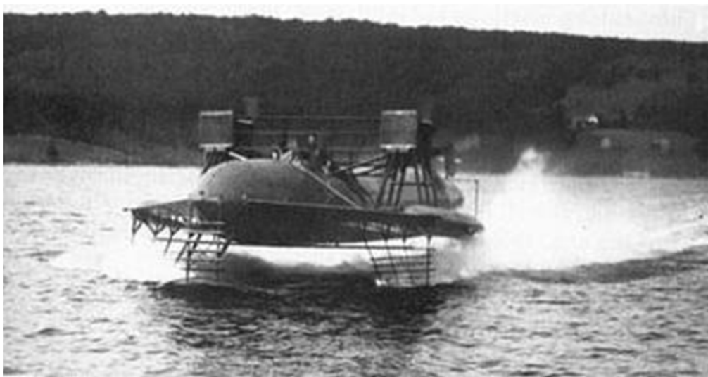
Fig. 1) Hydrofoiling has been around since the late eighteen hundreds (historic image with ladder foil configuration).
