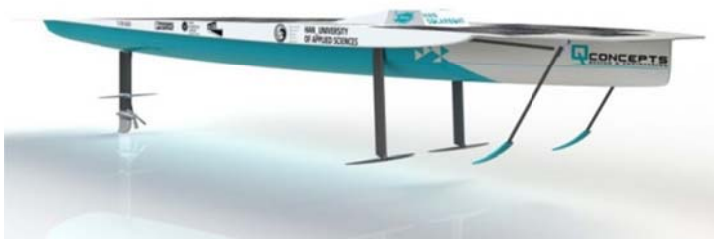
Fig. 3) Submersed foils configuration – with active lift control (mechanical) HAN-Solar boat PwrdbbyQ.
